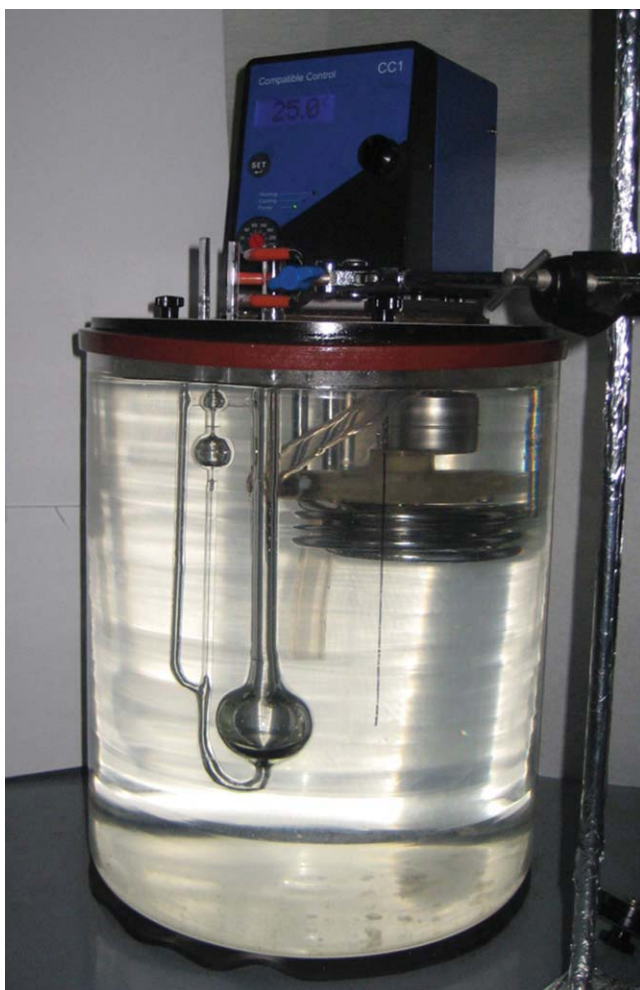
Figure 1 The photo of the equipment which is the home-made modified Ubbelohde-type capillary viscometer in a constant temperature bath. [Color figure can be viewed in the online issue, which is available at www.interscience.wiley.com .]
